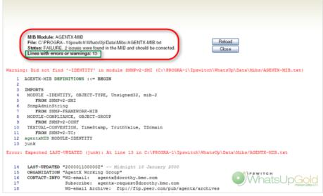
2 Now that the Viewer has helped you identify the problems in the code, open a text editor and correct the code. The MIB files are located in . . \Program
