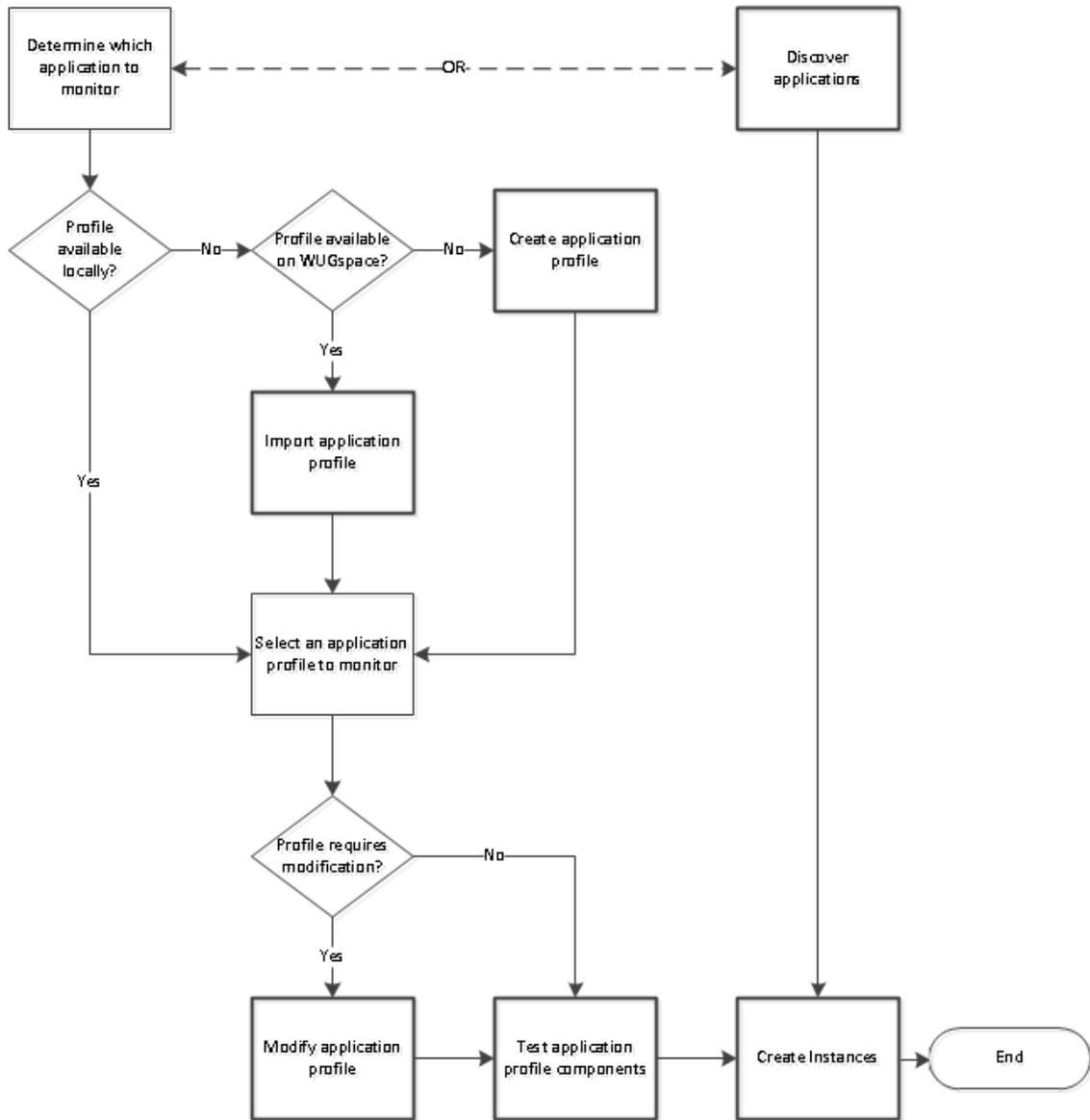
Refer to the table below for step-by-step instructions for each configuration process in the flow chart.
