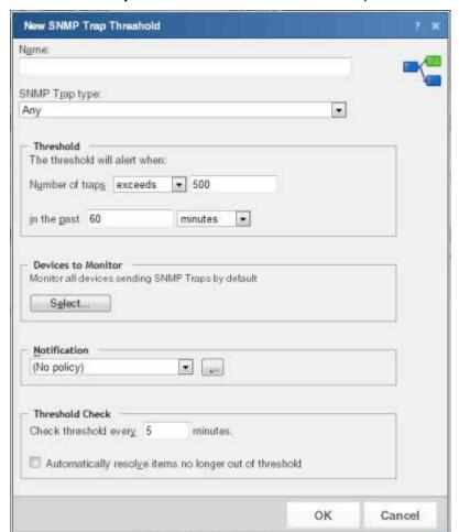
3 Select **SNMP Trap**, then click **OK**. The New SNMP Trap Threshold dialog appears.
