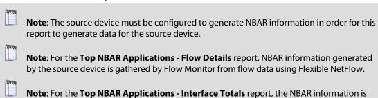
**Note**: For the **Top NBAR Applications - Interface Totals** report, the NBAR information is gathered from the source device using SNMP polling. The **Poll source for NBAR information** option is available on the Flow Source dialog.
