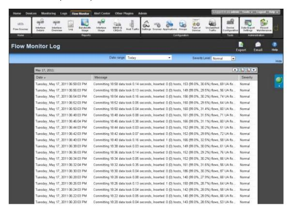
Each entry shows the date logged, the message about the activity, and the severity of the entry.
