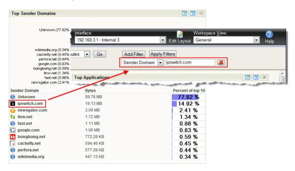
If you are viewing the Flow Interface Details report with a filter applied, clicking a link in a dashboard report refreshes the report with the selected data applied as an additional filter (the previously applied filters remain).
