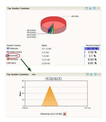
Several keyword filters coincide with more than one dashboard report and more than one time graph is displayed after the filter is applied. You can easily distinguish which dashboard reports in the Interface Details report are displaying time graphs by looking for the applied filter's name in parenthesis next to a report name.
