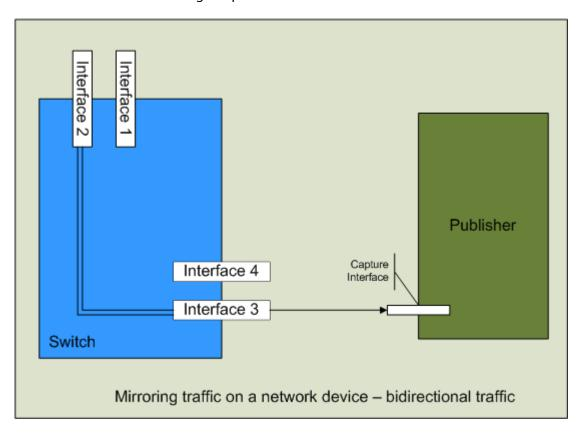
In the above figure, a single bidirectional traffic source has been created and mirrored to Interface 3. This traffic source contains all of the traffic received by and transmitted from Interface 2 combined. This combined bidirectional traffic is then sent to a single capture interface on the Flow Publisher.
