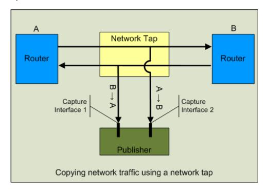
To configure each capture device correctly, you must identify an inbound and outbound interface. An interface identifier can be the pseudo-interface, the SNMP index, or an identifier you create and assign to the interface. The default setting is for the pseudo-interface value to be used as both **In Interface** and **Out Interface**.
