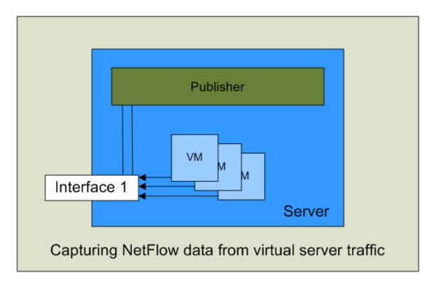
You can also collect NetFlow statistics on a virtual server by installing NetFlow on the virtual server and configuring the capture mode of the virtual interface to Normal. This configuration will provide NetFlow statistics on all of the traffic to or from the virtual server.
