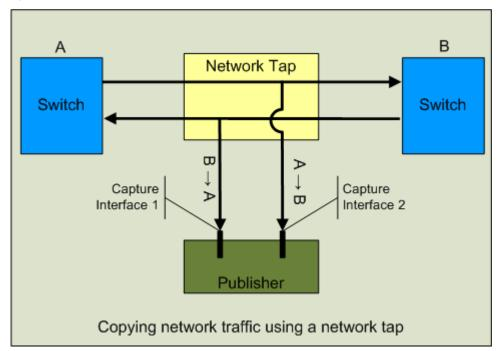
When you use a network tap to copy traffic to the Flow Publisher, you need to install a network tap in the segment that carries the traffic you want to capture. Next, connect the outputs from the tap directly to the capture interfaces on the Flow Publisher. The network tap will copy the full-duplex traffic and send traffic from each direction on a separate connection to two seperate capture interfaces on the Flow Publisher.
