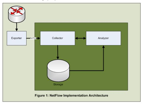
The exporter can be either an included function of the network device, such as the NetFlow export functionality on Cisco routers, or it can be an external publisher configured to monitor one or more interfaces on the device, such as the WhatsUp Flow Publisher.
