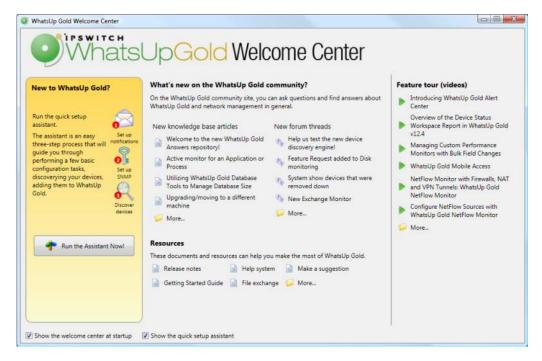
Most importantly, the Quick Setup Assistant collects information about your SNMP communities. The Quick Setup Assistant automatically generates SNMPv1 and SNMPv2 credentials for each community entered.
